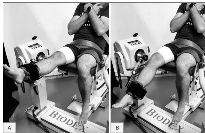
Figure 2. JPS procedures for the SIT_ECC test: (A) describes the starting position (full knee extension), and (B) the leg positioned at the target angle (45° of knee flexion).
