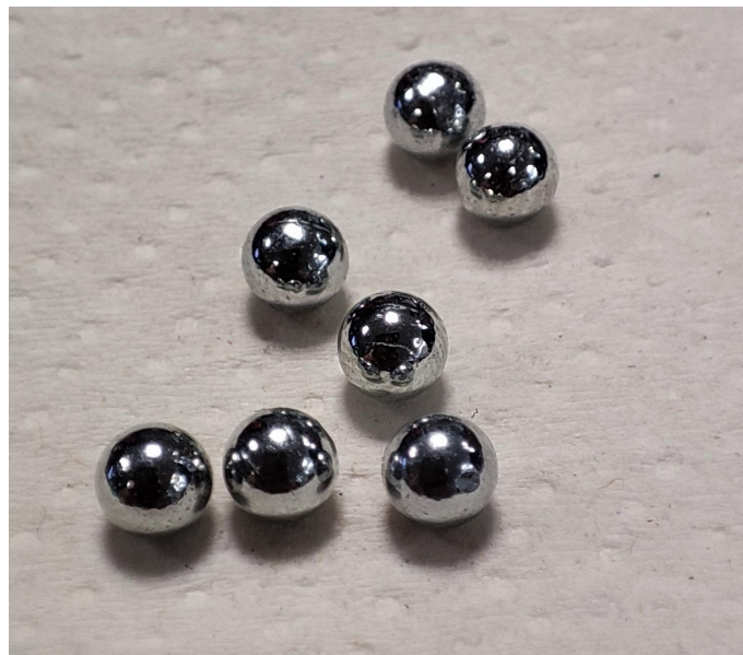
Figure 4.24: Steel spheres of 4.5 mm.
