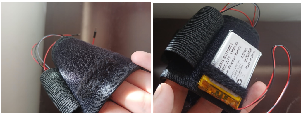
Figure 4.11: Demonstration of the sewn clothstrap, stabilizing the battery in the bracelet.
