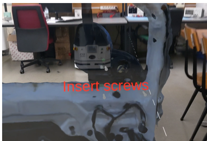
Figure 4.20: Prompt in Virtual Mode guiding the user to insert holographic screws in HoloLens deployment.
