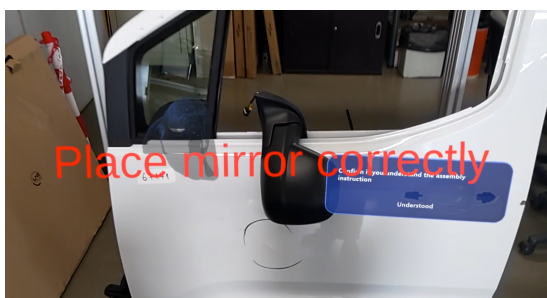
(a) Text feedback when the mirror is incorrectly placed in Full Mode.
