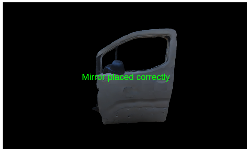
Figure 4.6: Text feedback in Unity's Play Mode for correct mirror placement
