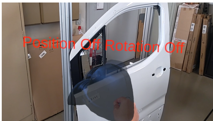
Figure 4.24: Mirror placement guided by ghost hologram and text feedback in Mixed Mode.
