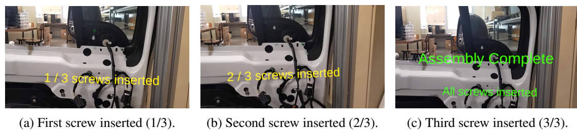
Figure 4.35: Text feedback in Full Mode when screws are inserted in HoloLens deployment: (a) first screw, (b) second screw, and (c) all screws inserted.
