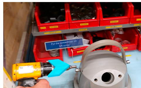
(b) MR instructions guiding the operator through the assembly process.
