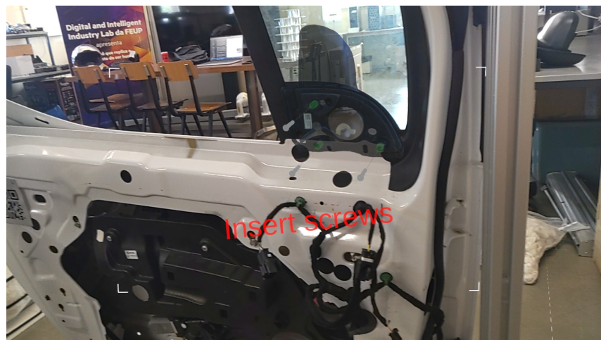
Figure 4.26: Prompt in Mixed Mode guiding the user to insert holographic screws in HoloLens deployment.
