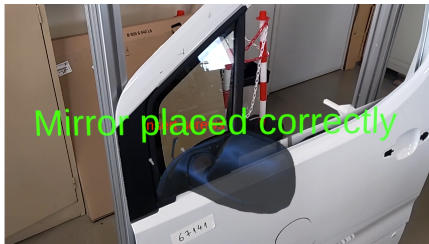
Figure 4.25: Text feedback in Mixed Mode for correct mirror placement in HoloLens deployment.
