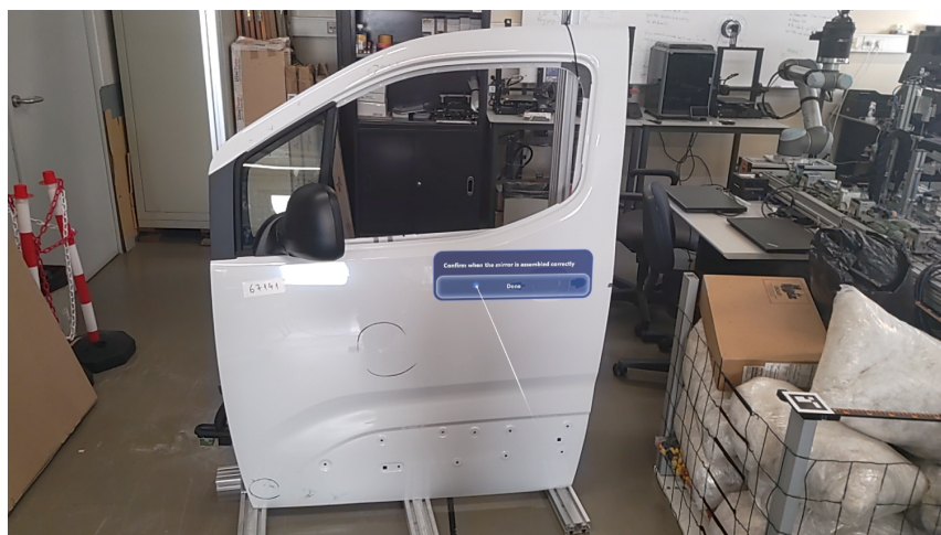
Figure 4.31: User confirming they have placed the mirror via dialog in Full Mode within HoloLens deployment.
