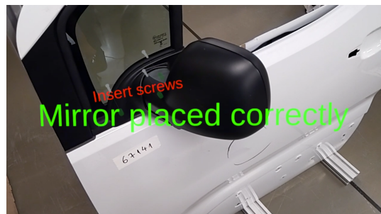
(b) Text feedback when the mirror is correctly placed in Full Mode.
