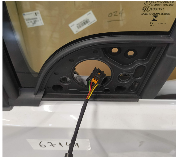
Figure 3.4: Correct cable position, passed through the attachment piece on the quarter glass.
