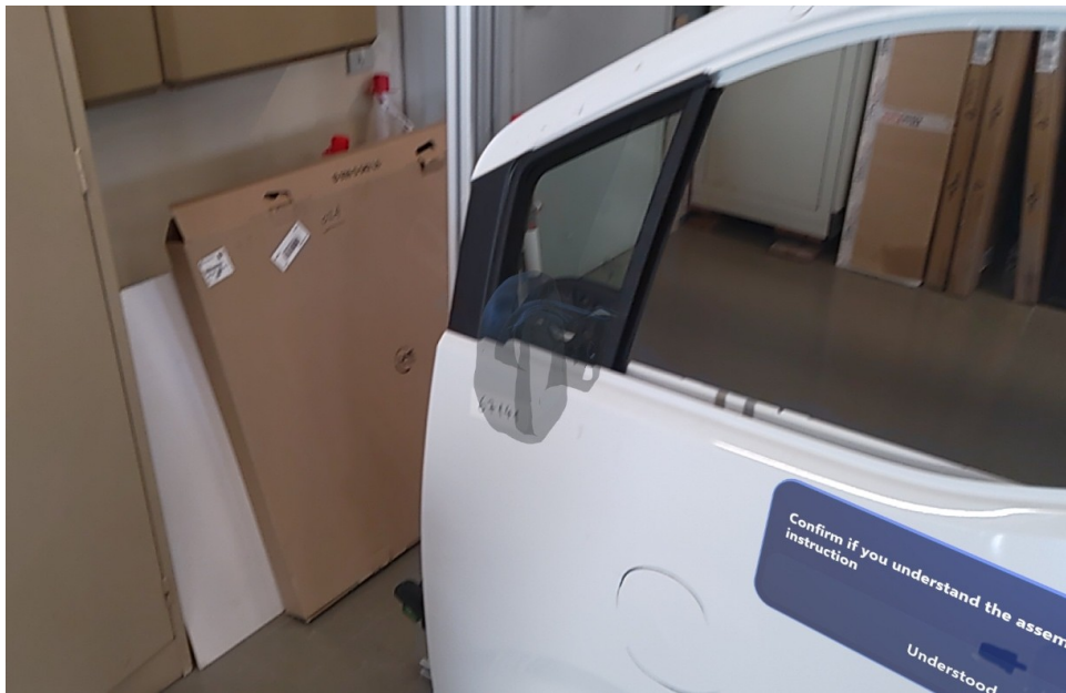
Figure 4.36: Example of misalignment: the mirror ghost hologram appears offset from the actual mirror position in Full Mode.
