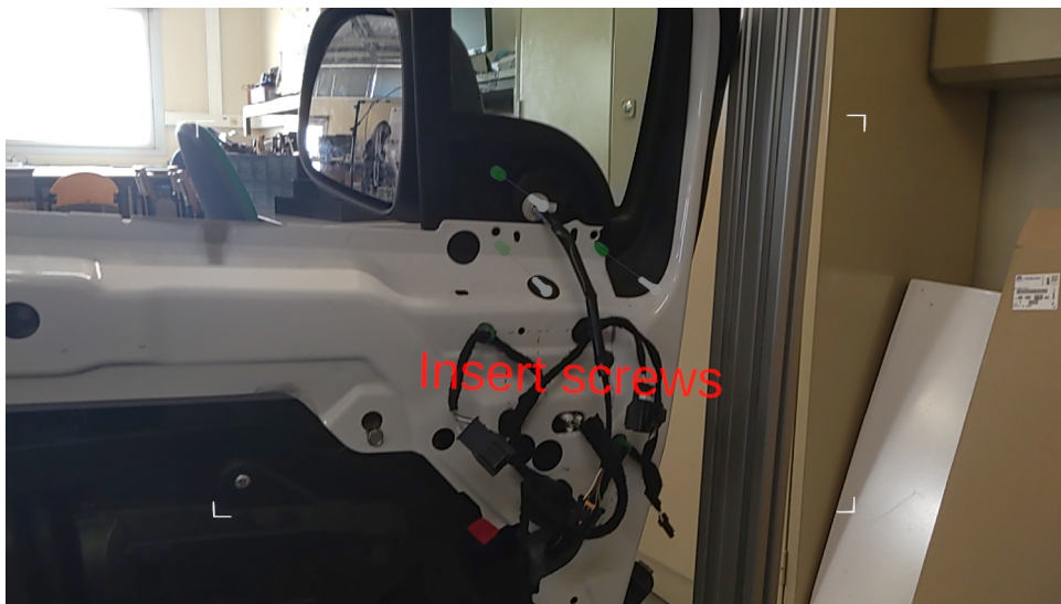
Figure 4.37: Example of misalignment: the holographic screws do not perfectly align with the physical holes in Full Mode.
