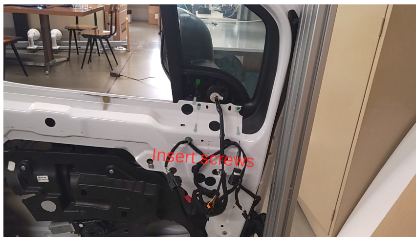
Figure 4.34: Prompt in Full Mode guiding the user to insert holographic screws in HoloLens deployment.
