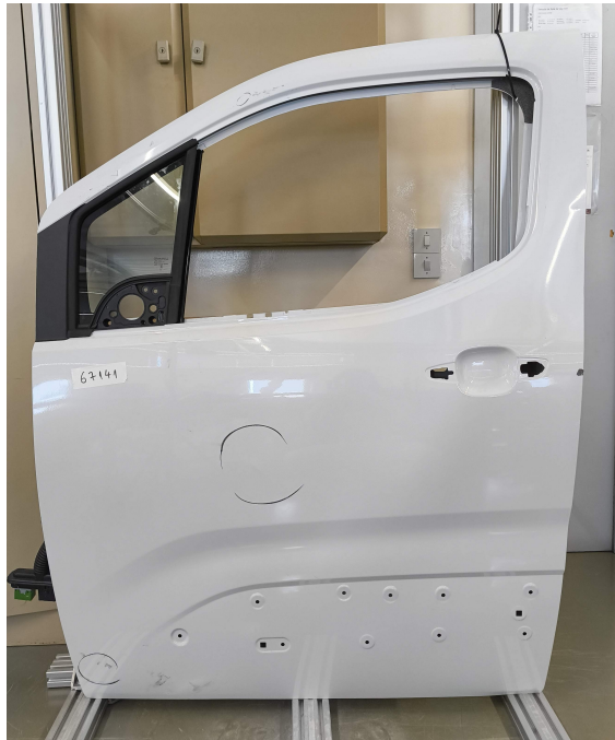
Figure 3.3: Van door with quarter glass piece installed
