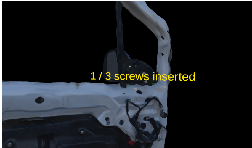
Figure 4.8: Text feedback in Unity's Play Mode when one out of three screws is inserted.
