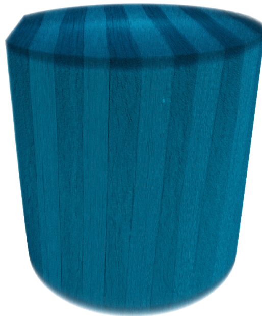
Figure 4.46: 3D rendering of the undamaged volume scanned for the [2T/H/2T] specimen, showing the uniform layered microstructure.
