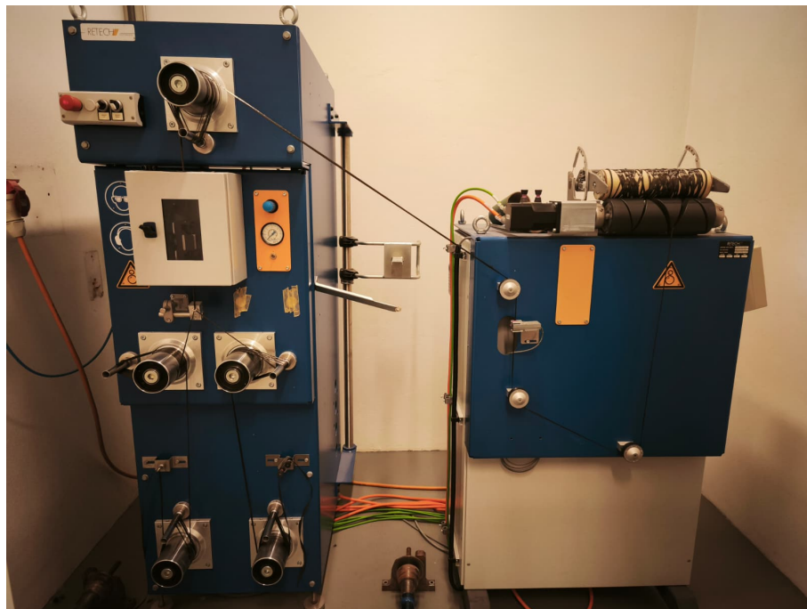
Figure 3.2: The Retech air-jet co-mingling experimental setup.
