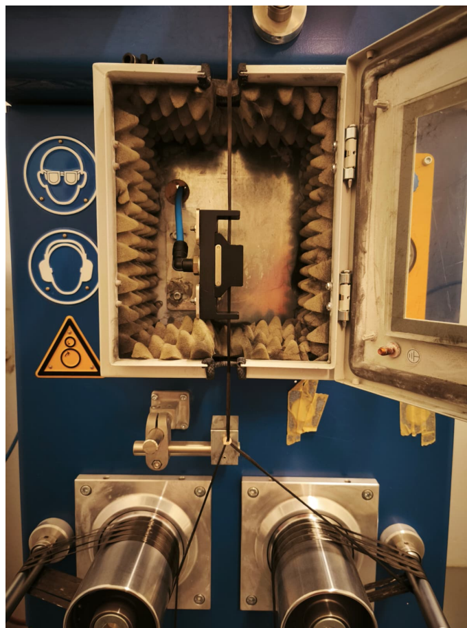
Figure 3.4: The air-jet mixing zone, showing the feed godet sets, the merging guide, and the open mixing box containing the nozzle.
