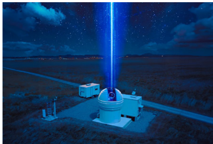
Figure 2.1: ONERA’s optical ground station FEELINGS established a stable two-way laser link with the Airbus Defence and Space TELEO payload in geostationary orbit (ONERA 2024).
