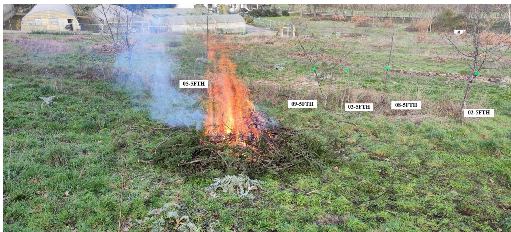
Figure 5.2: Five sensor modules acquire data of fire ignition in the first scenario with low TCD.
