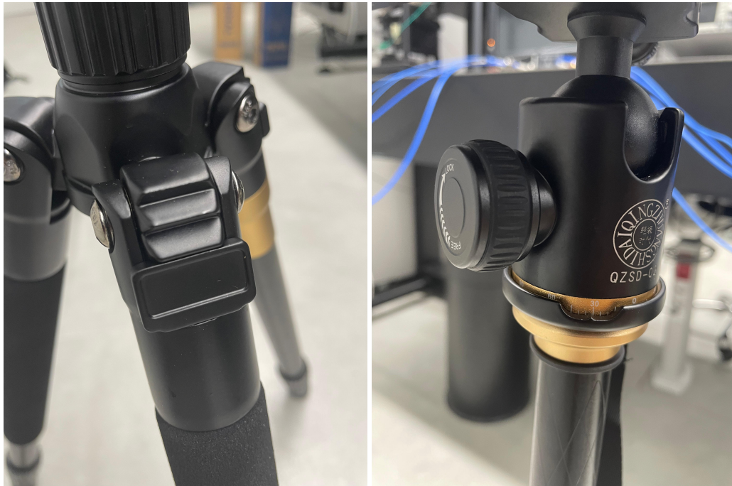
Figure 3.20: Detail of the tripod leg adjustment for precise leveling of the antennas.
