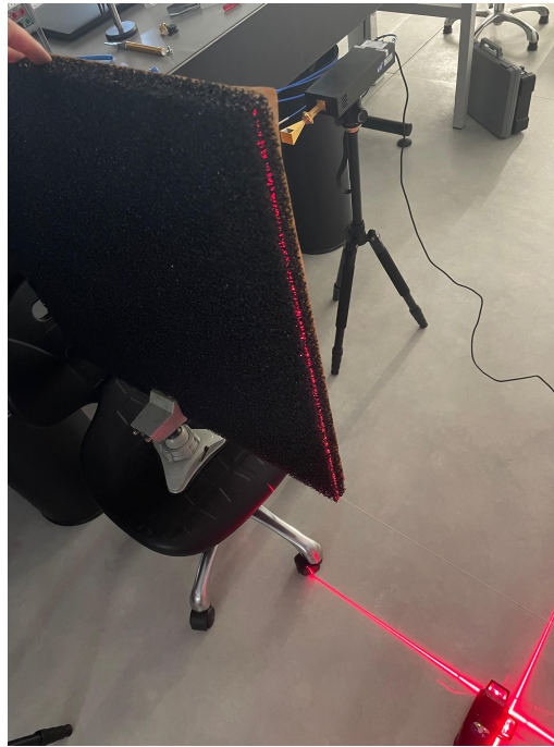
Figure 3.21: Alignment of the absorbing sample in the perpendicular incidence configuration.
