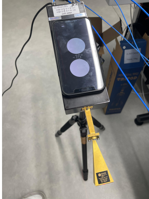
Figure 3.19: Reading the angle of inclination of the antenna using a mobile application.
