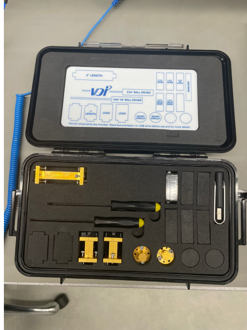
Figure 3.2: SOLT calibration kit used to calibrate the measuring system in the plane of the WR10 extender connectors.
