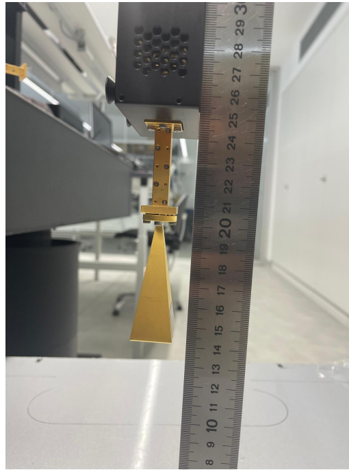
Figure 3.13: Checking that the physical distance between the sample and the antenna's radiation point is compatible with the measured time.
