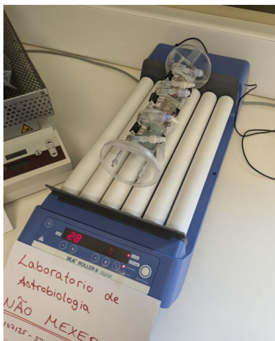
Figure 15. 2-D clinostat adapted for bag bioreactors, used for simulated microgravity experiments.
