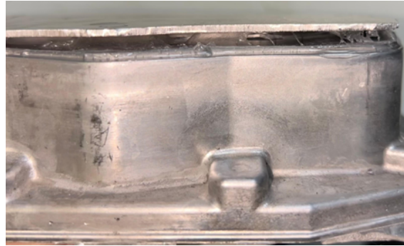
Figure 11: Failure mode of the LS-XU adhesive in internal pressure testing.
