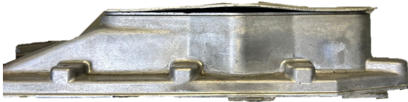
Figure 58: Failure mode of the FSW specimen in internal pressure testing.
