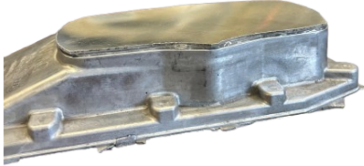
Figure 16: Specimen prepared for the internal pressure test with LS-XU adhesive.
