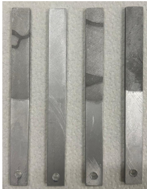
Figure 4: Different results of the anodization of as-cast aluminium substrates.
