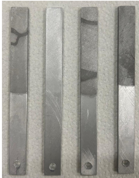
Figure 13: Different results of as-cast aluminium substrates anodization.
