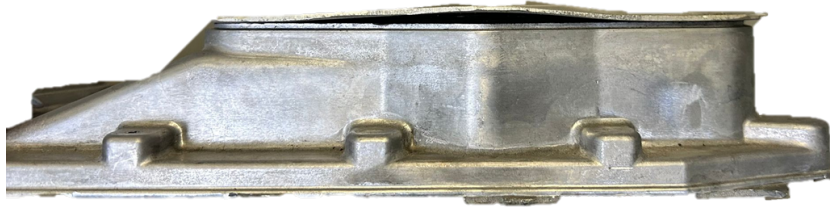
Figure 13: Failure mode of the FSW specimen in internal pressure testing.
