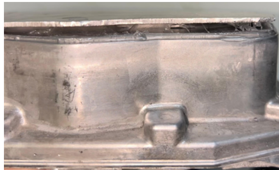
Figure 56: Failure mode of the LS-XU adhesive in internal pressure testing.
