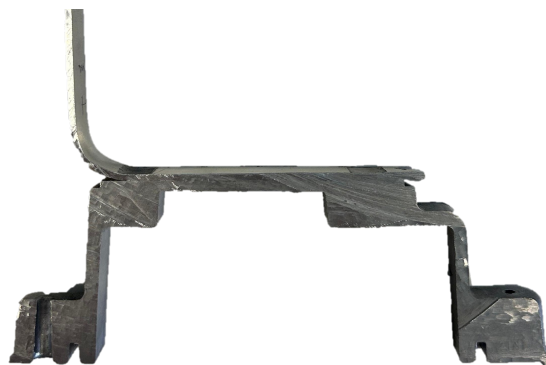
Figure 15: 90° peel test specimen with FSW.
