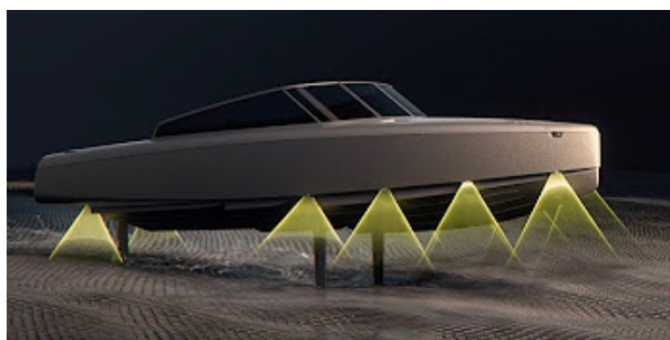
Figure 2.27: Candela depth sensor scheme, [42].
