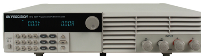
Figure 7.3: BK Precision 8510 DC Electronic Load used for programmable discharge testing, from [57].
