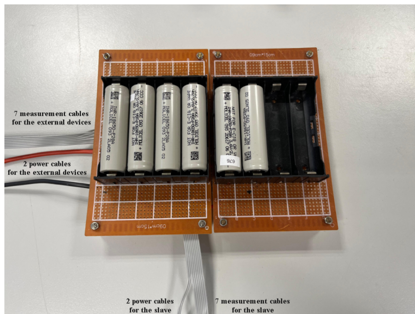
Figure 6.1: Assembled 6-cell battery pack.
