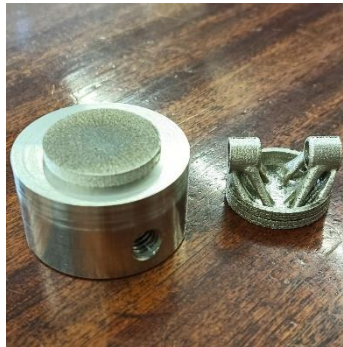
Figure 86: Optimised piston separated from the LPBF base.
