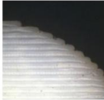
Figure 13: Stair casing effect [78].
