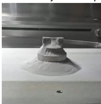
Figure 84: Optimised piston covered with unfused powder in LPBF.
