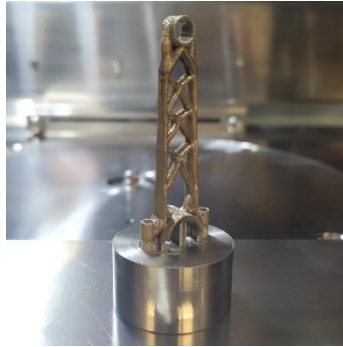
Figure 88: Cleaned, optimised connecting rod fused to the LPBF base.
