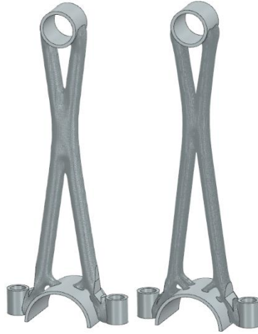
Figure 56: Optimised connecting rods with medium resolution (left) and maximum resolution (right).
