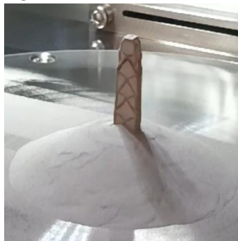
Figure 87: Optimised connecting rod covered with unused powder in LPBF.
