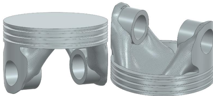
Figure 44: Third version of the optimised piston.
