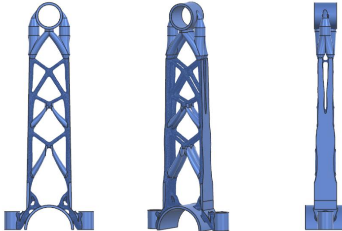
Figure 80: Views of the final version of the optimised connecting rod.
