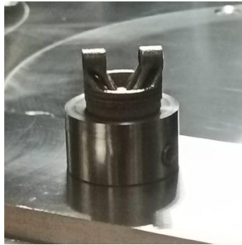
Figure 85: Cleaned, optimised piston fused to the LPBF base.
