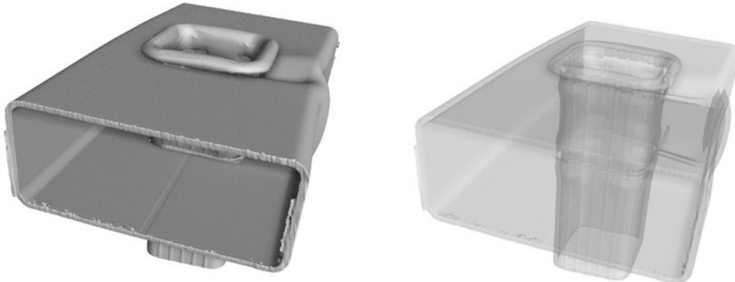
Figure 21: CT images of the DA2.58 profile (185 °C, 6 hours and 58 mm).
