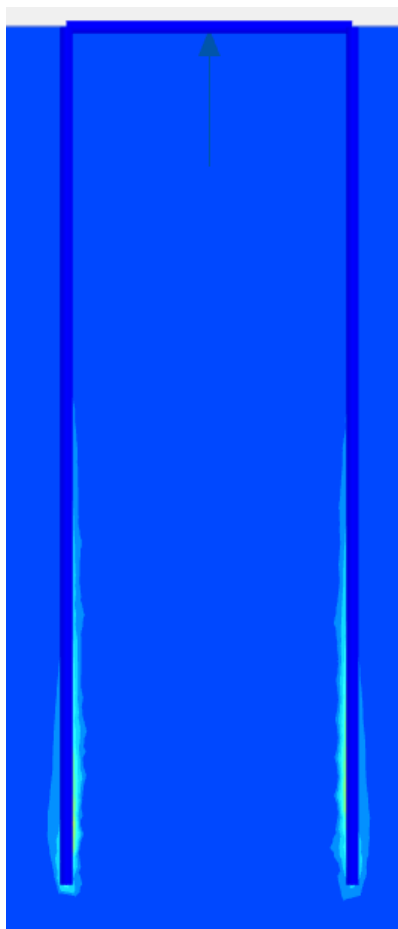
Figure 6.12 – Total deviatoric strain of a suction caisson in plane strain model under a uplift load
