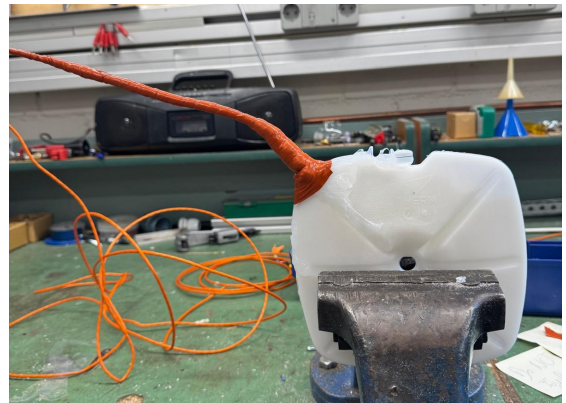
Figure 6.4: Final Capsule RTD Insulation.
