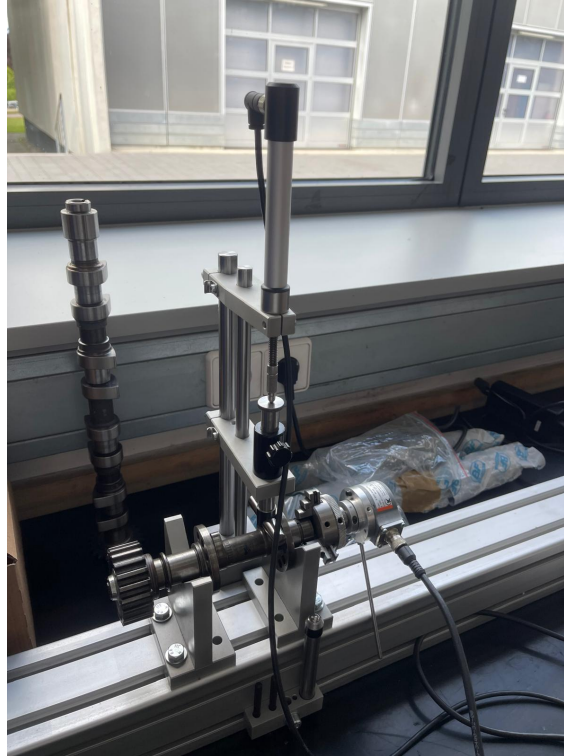
Figure 4.28: Setup for measuring the camshafts' lift curves
