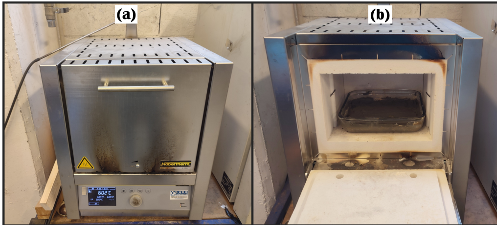
Figure A.2: Nabertherm L 9/11 muffle furnace (a) closed; (b) open, with a sludge sample inside.
