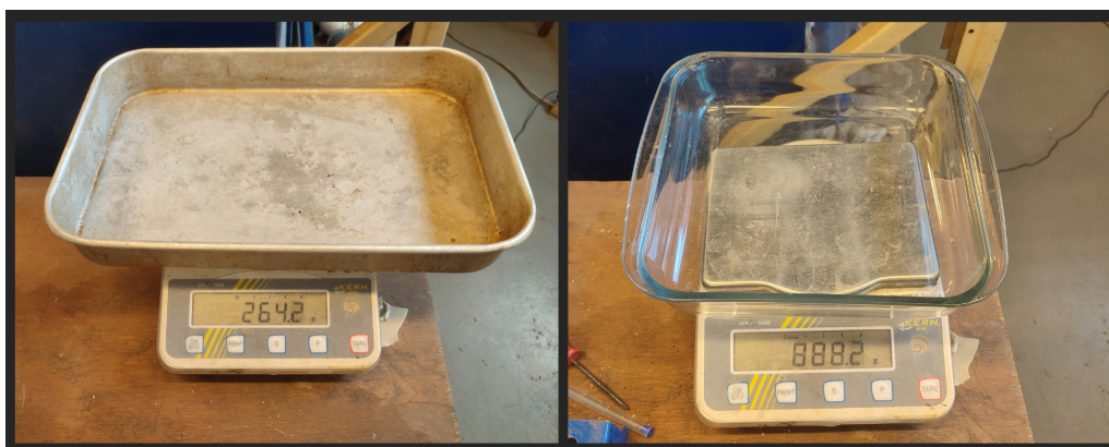
Figure A.3: Steel and glass trays used in the sludge drying experiments.
