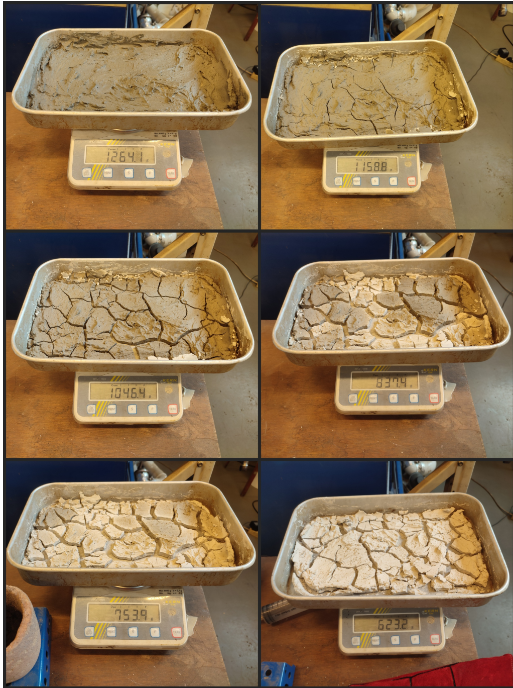
Figure A.7: Sample photographs along the 100 °C FC experiment. MC are as follows (from left to right, top to bottom): 65.25 %, 61.16 %, 55.57 %, 39.38 %, 29.04 %, and 3.20 %, respectively.
