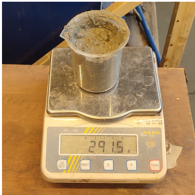
Figure A.6: Plastic beaker measuring the mass of 250 mL of wet sludge.
