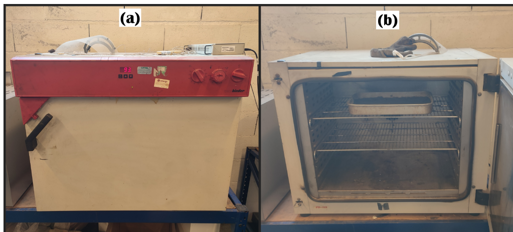
Figure A.1: BINDER FD115 FC oven (a) closed; (b) open, with a sludge sample inside.
