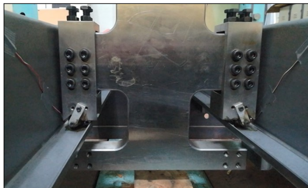
(a) Load actuator placed on top of the lower flange (downward load case).
