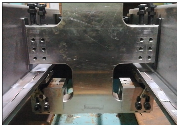
(b) Load actuator placed underneath the lower flange (upward load case).
