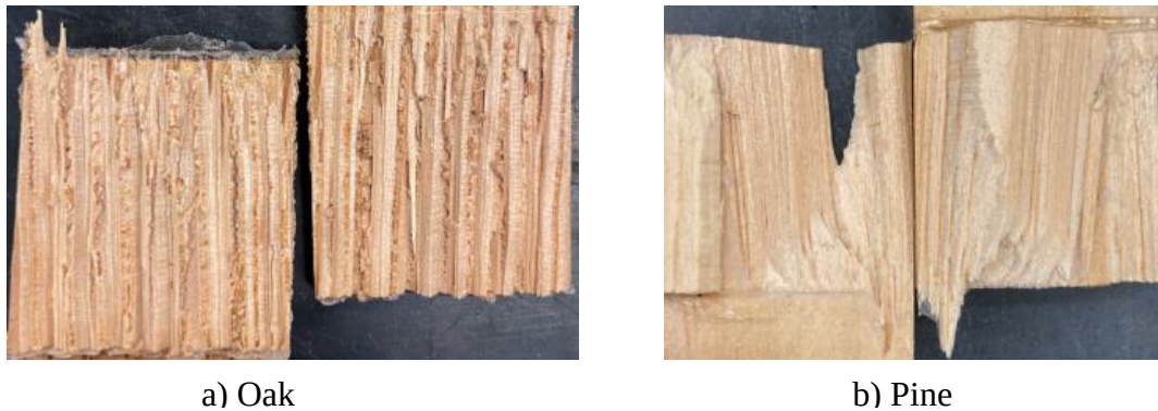
Figure B. 23: Failure modes obtained for reference joints under impact conditions.
