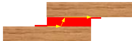
Figure B. 21: Crack path scheme for both toughened configurations under quasi-static conditions
