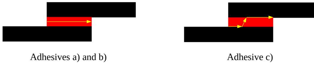
Figure A. 24: Crack path scheme for the three different adhesives under impact and high temperature conditions – a) Zeon LS-XU; b) AF 163-2k; c) Nagase Denatite
