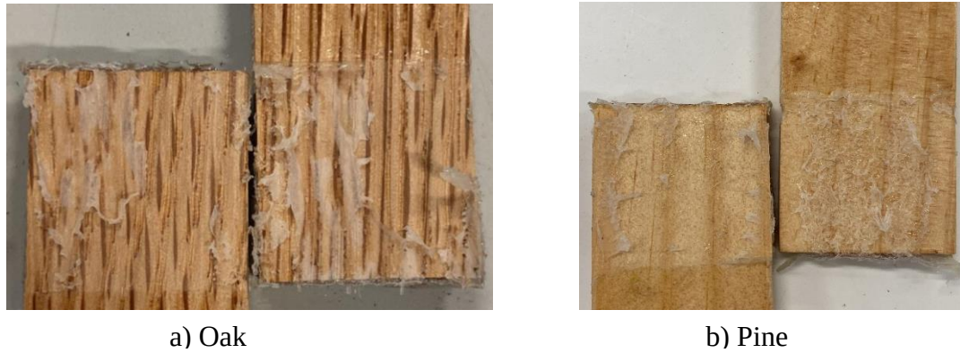
Figure B. 20: Failure modes obtained for toughened joints under quasi-static conditions
