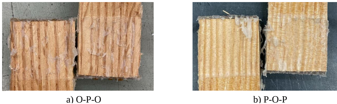
Figure B. 26: Failure modes obtained for hybrid joints under quasi-static conditions.
