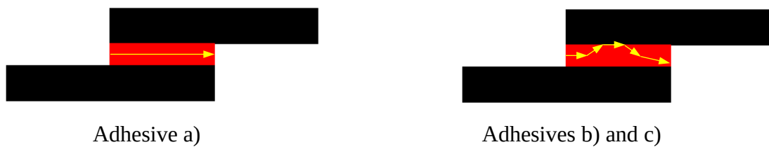
Figure A. 21: Crack path scheme for the three different adhesives under quasi-static and high temperature conditions – a) Zeon LS-XU; b) AF 163-2k; c) Nagase Denatite
