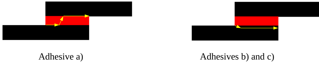
Figure A. 8: Crack path scheme for the three different adhesives under impact and room temperature conditions – a) Zeon LS-XU; b) AF 163-2k; c) Nagase Denatite
