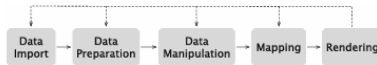
Figure 3.1: The data visualization pipeline, illustrating the transformation of raw data into structured visual formats.
