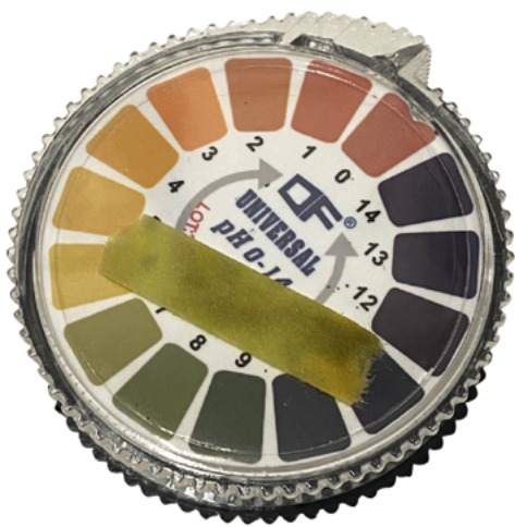
Figure 14- pH strip reading target range (neutral to alkaline)
