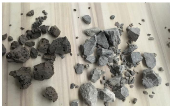
Figure 14. SS (left) and NA (right) aggregate
