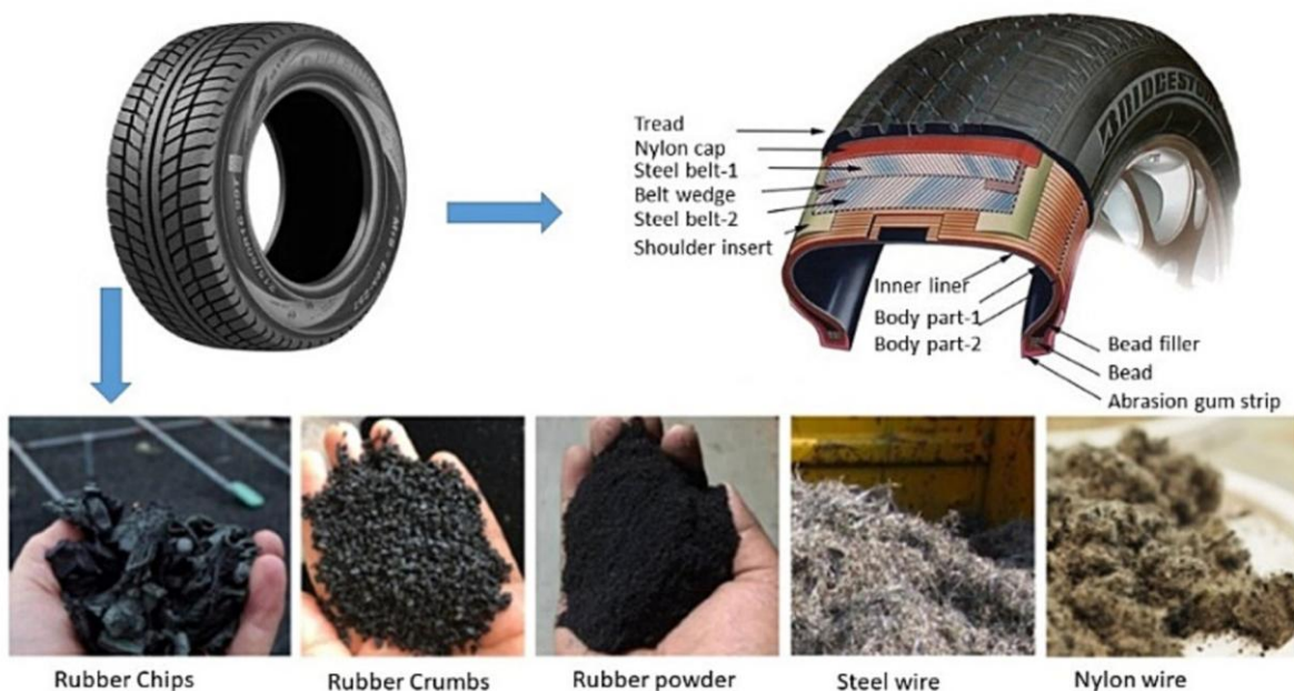
Figure 16. Various recycled materials extracted from waste tyres [71]
