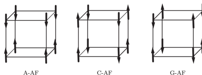
Figure 2.2: Three types of antiferromagnetic (AF) structures, A- AF, C- AF, and G- AF.
