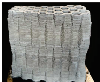
Lightweight concrete wall [9]
