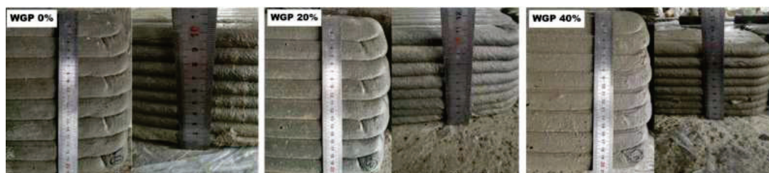
Waste glass powder in geopolymers concrete [116]
