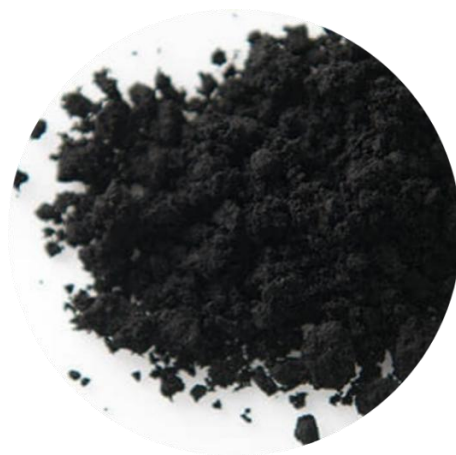
Figure 3.2. Pt5/AC from Sigma-Aldrich in powder form.
