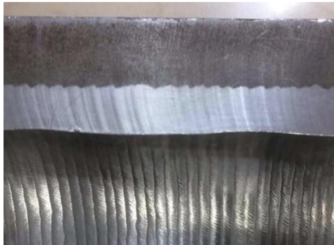
Figure 2. Low alloy steel pipe cladded with Inconel 718
