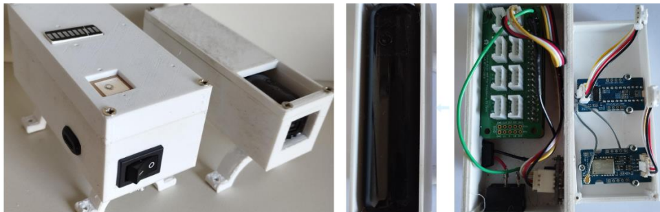
Figure 4.5: 3D-printed case containing the electronics and internal wiring.
