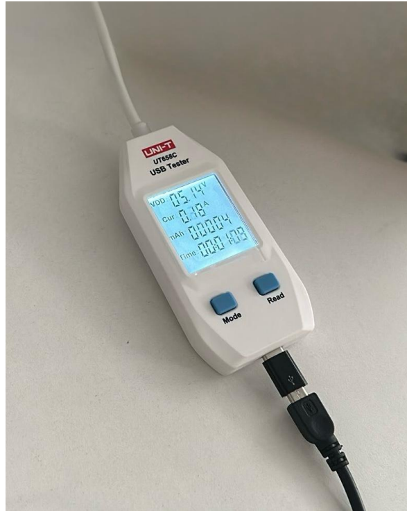
Figure 5.5: Uni-T UT658C used to measure current during operation of the system.
