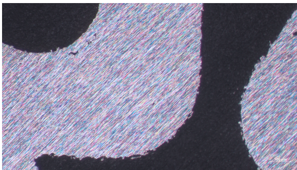
(e) S38: P = 210 W, v = 600 mm/s, d = 85 \mu m, E = 61.68 J/mm 3
