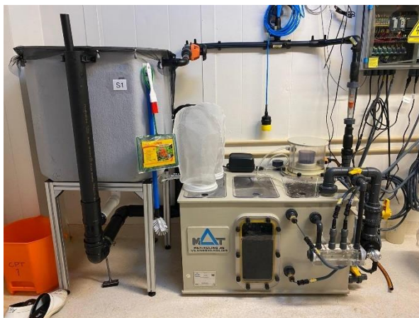
Figure 4 - Picture of one of the Lab scale RAS.
