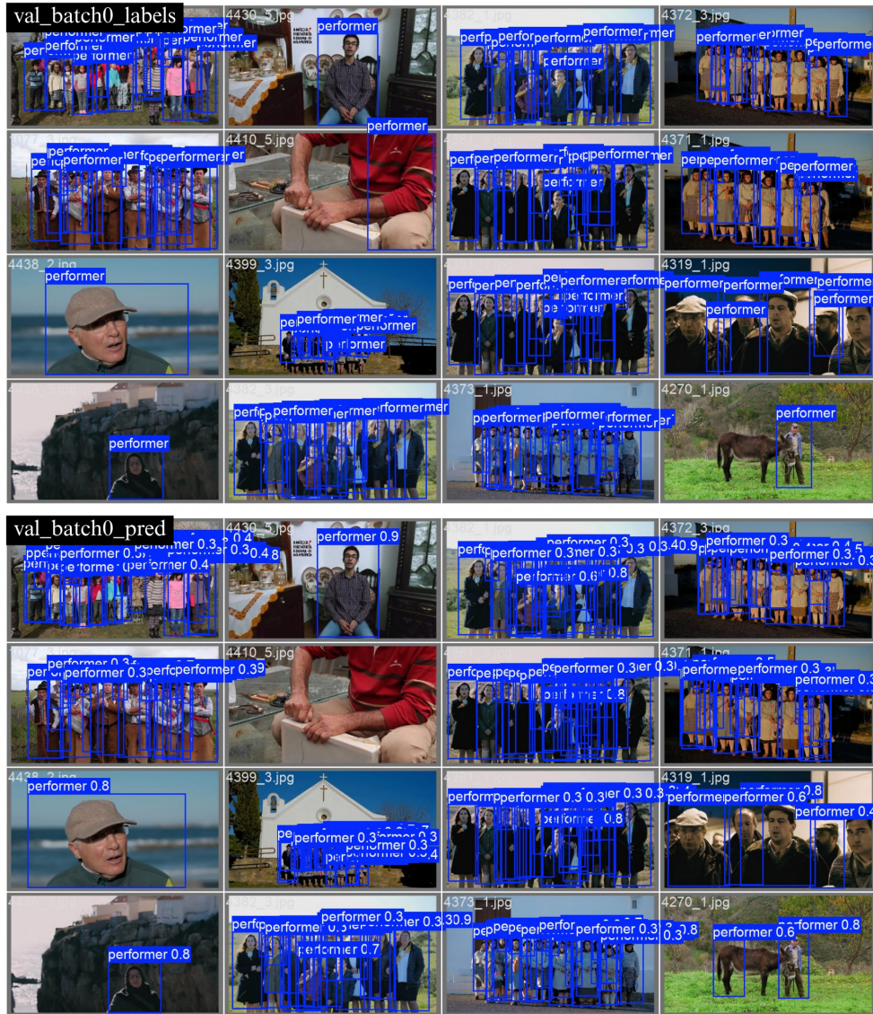
Figure 4.7: Qualitative analysis of model performance on a sample validation batch. The top panel shows the ground truth labels, while the bottom panel shows the corresponding predictions from the YOLOv11s model, including confidence scores. This comparison highlights successful detections as well as challenges such as missed performers in dense crowds and lower confidence scores in complex scenes.
