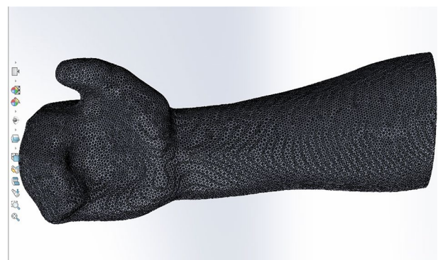
Fig. 7 Imported mesh file of the scanned hand in SOLIDWORKS software
