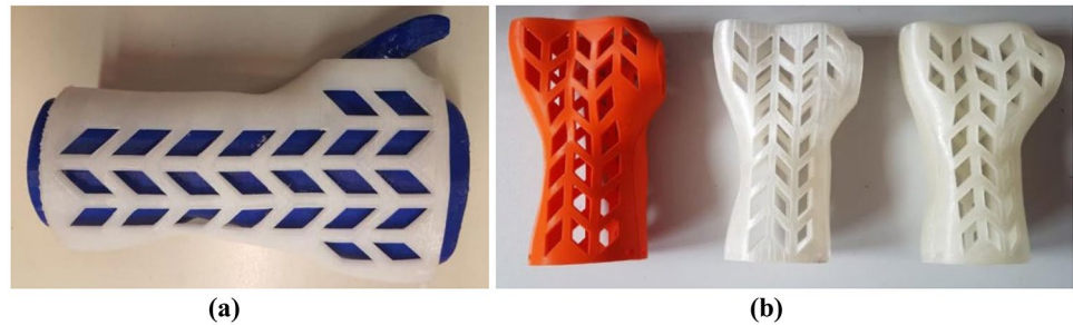
Fig. 1 RO modelling results. a ORTHOSIS on the forearm phantom, b vertically manufactured orthosis using the PLA material with different strategies [(left to right): economical, accurate, strong] [28]
