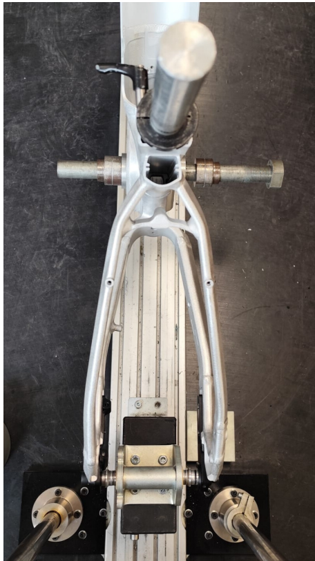
(a) Hinge feature at rear dropouts
