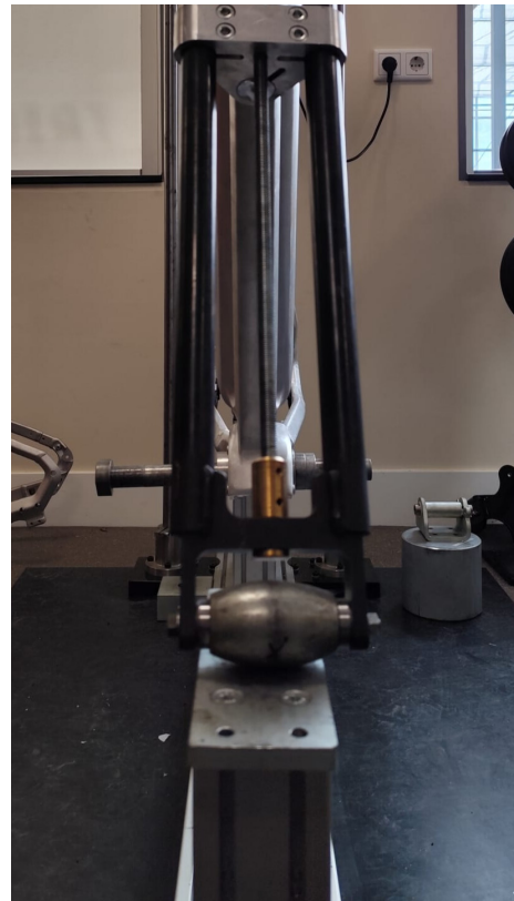
(b) Steel anvil plate fixture
