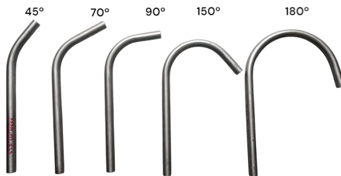
Figure 3.9: Tube with the five angle that will be analysed. In order: 45°, 70°, 90°, 150°, 180° (Example of the figure: SS304 thickness=1.5 mm CLR120)
