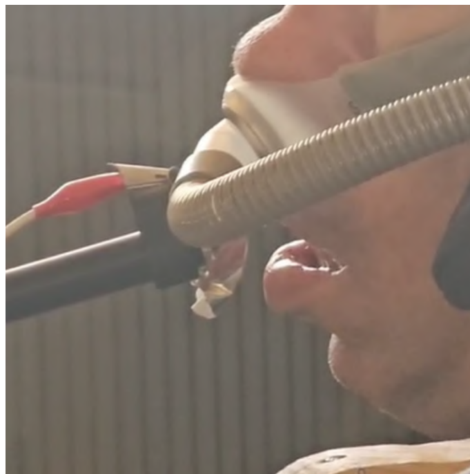
Figure A.11: Lips Interface, triggers when the lips enter in contact with the aluminum piece
