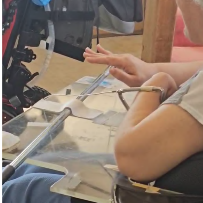
Figure A.10: Tube and Triangle Interface, Triggers when hand touches the tube
