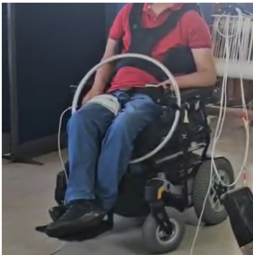
Figure A.6: Circumference Interface, triggers when hand rests on circular metal bar
