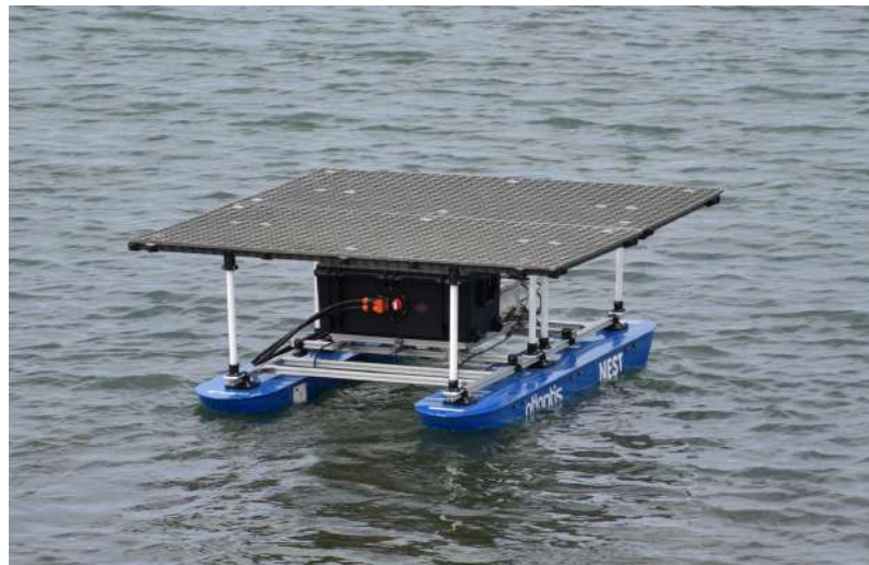
Figure 3.2: NEST USV, featuring a catamaran design and a 2×2 meter UAV landing platform for autonomous inspection operations.
