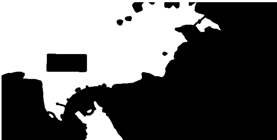
Figure 4.9: Final navigable map after applying dilation for safety margins, ensuring a safe distance from shores and static obstacles.
