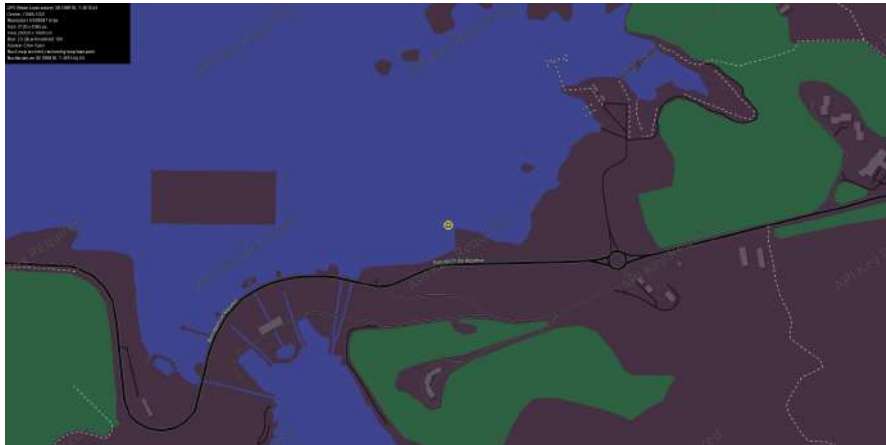
Figure 4.7: Raw mission map downloaded from the OpenStreetMap API, showing the NEST's position (yellow \oplus ) and metadata for debugging.
