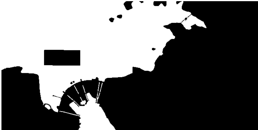
Figure 4.8: Binary threshold of the raw map after pre-processing. Water areas are preserved as navigable zones, while land is filtered out.
