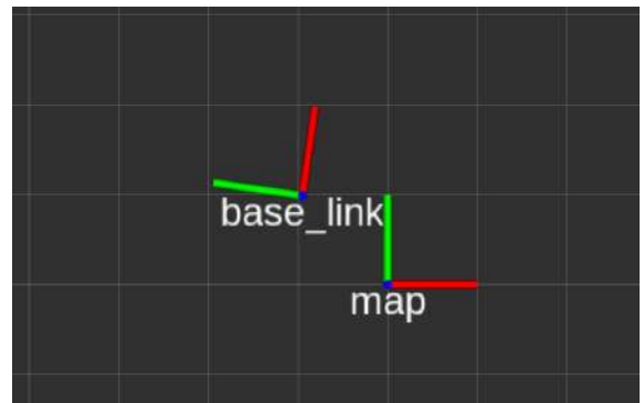
Figure 4.2: Representation of the base_link and map frames in the RViz tool.
