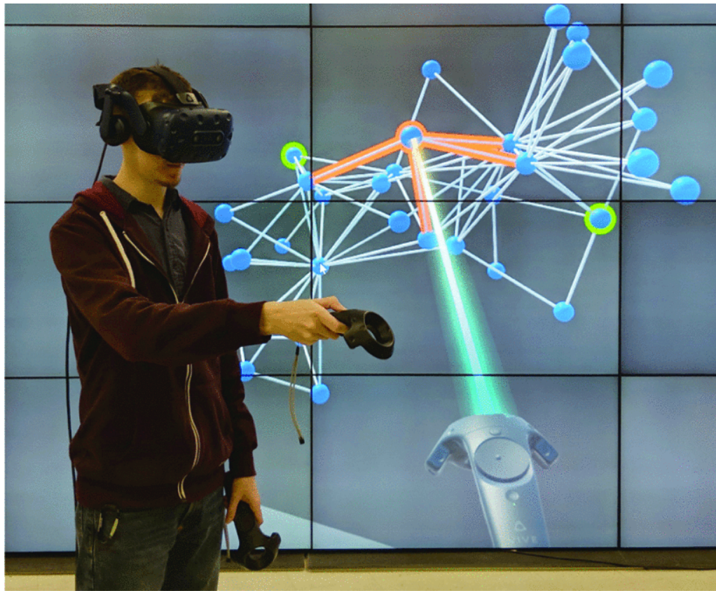
Figure 2.6: A user interacts with an immersive 3D network visualization using a head-mounted display and controllers. A virtual laser pointer is implemented to highlight and select nodes. Users can scale and relocate the network using pinch-to-zoom interaction with both controllers. The figure shows the karate network in a 3D layout [23].
