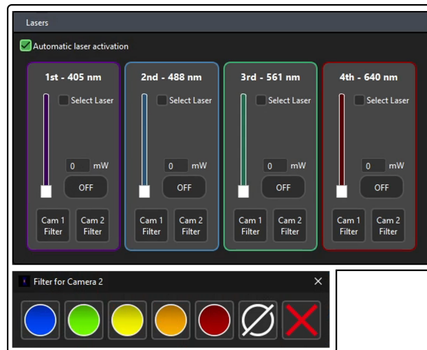
FIGURE 3.4: Lasers Widget of the VitaSlice software. It allows the user to control four independent lasers, including power adjustments via sliders and on/off toggles. For automated acquisition, each laser must be paired with the appropriate emission filter. The assignment is done separately for each camera with dedicated buttons, which open the filter selection window shown below.
