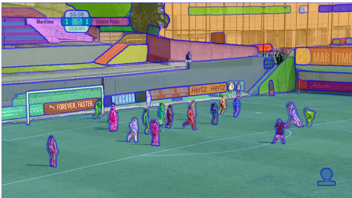
Figure 3.7: Full segmentation of a frame taken from a goal clip using SAM
