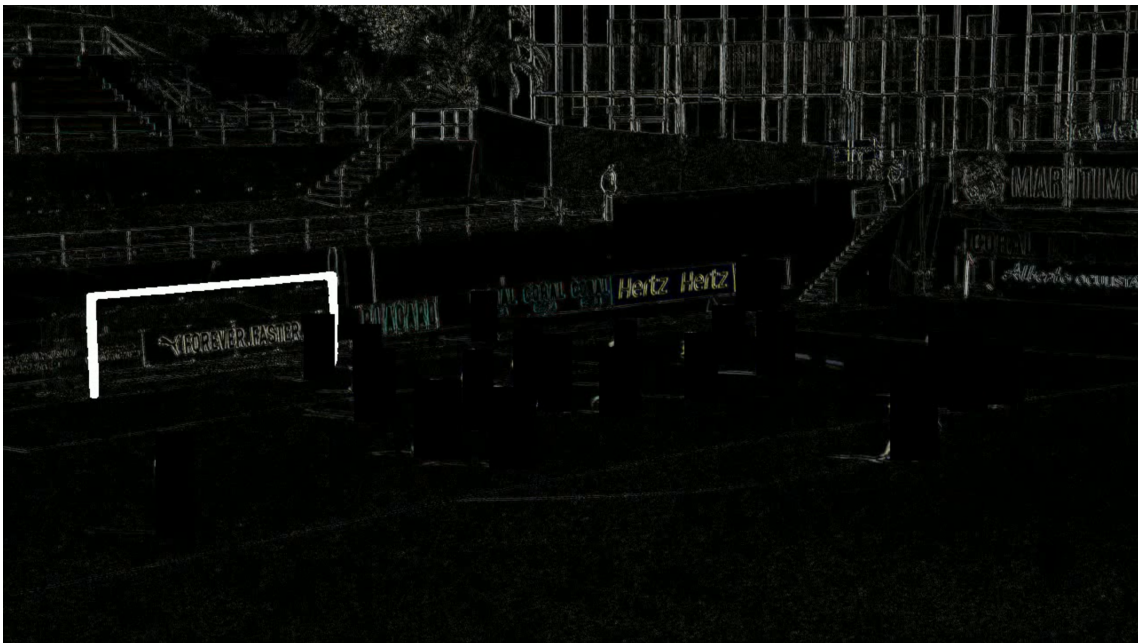
Figure 4.10: Frames Subtracted Video + Remove Players (YOLO) Bounding Box + Goalposts segmentation (YOLO + SAM). The predicted goal posts are marked white and the ball with heavy motion blur appears with two trails
