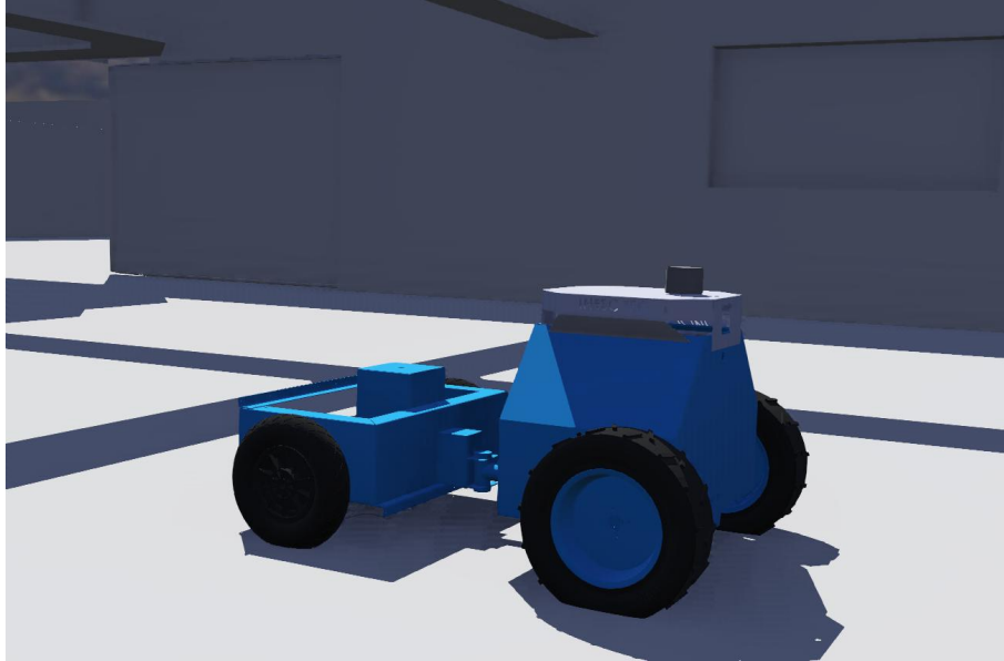
Figure 3.3: Rendered model of the Modular E robot used in simulation. The platform features a front-mounted sensor suite and a differential drive architecture.
