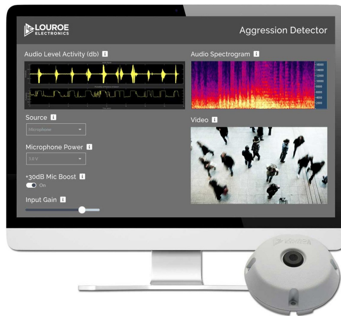
Figure 1.2: Example of an aggression detection interface used in urban surveillance systems. The system integrates real-time audio signal processing, including waveform monitoring and spectrogram analysis, with video feeds to detect and respond to hostile auditory events in public spaces. Source:[2]
