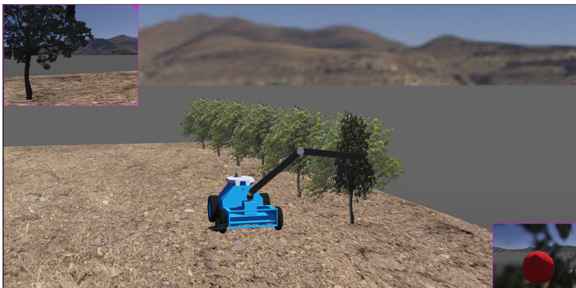
Figure 4.2: Simulation of the ArBeH manipulator in the Webots virtual environment and the displays of the views from the two onboard cameras.
