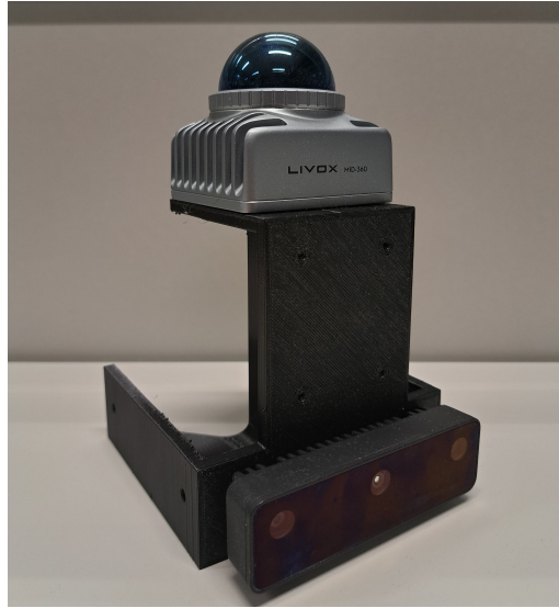
Figure 5.1: Setups of sensors used in data collection, including the OAK-D S2 RGB-D sensor and the Livox Mid-360 LiDAR sensor.
