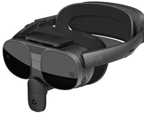
Figure 4.1: The Vive XR Elite headset with the Full Face Tracker accessory.
