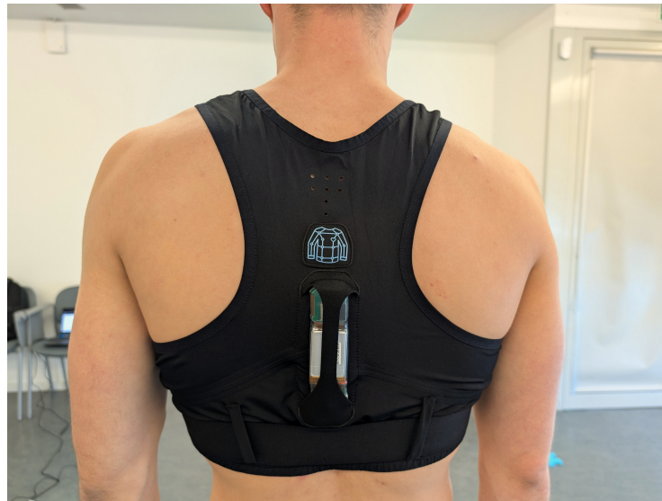
Figure 2.1: Prototype of the sensorized vest developed in the TEXP@CT project, highlighting the IMU and central sensor compartment.
