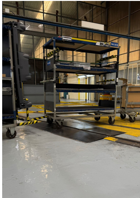
Figure 4.46: New ramp installed - smoother dolly transition
