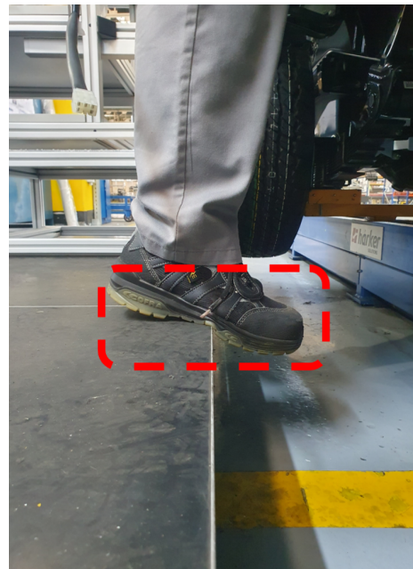
Figure C.29: Operator safety risk, when close to the car – need for additional step
