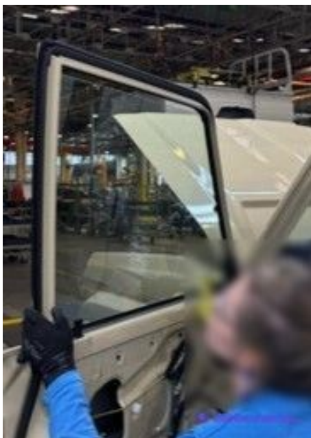
Figure B.23: Window cleaning and inspection
