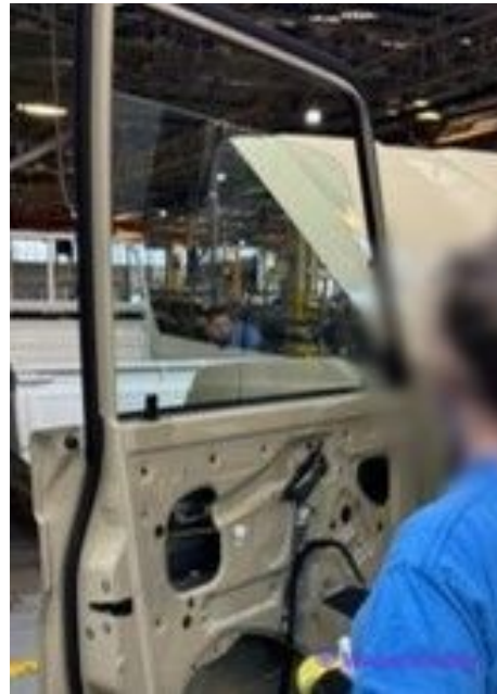
Figure B.22: Window functional testing
