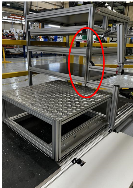
Figure 4.38: New lock mechanism for step (open position)
