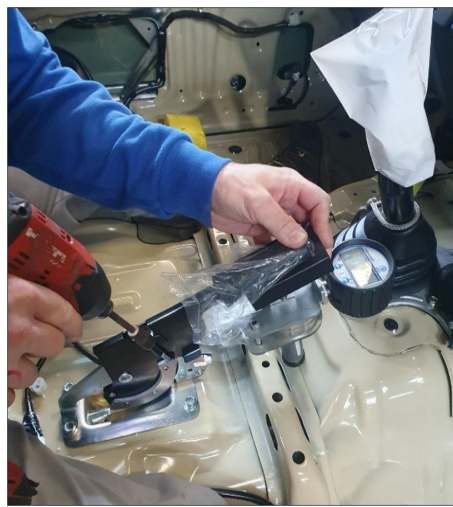
Figure 4.48: Handbrake assembly with measuring instrument in use
