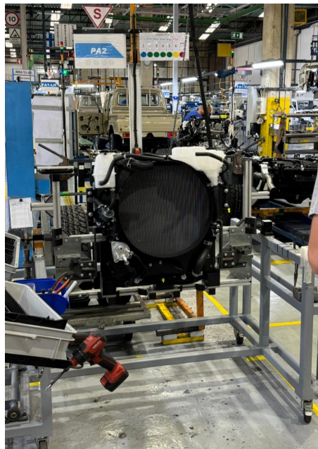
Figure 4.42: Radiator pre-assembly station
