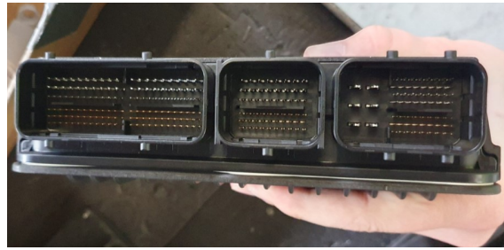
Figure 4.43: ECU stored with no protections
