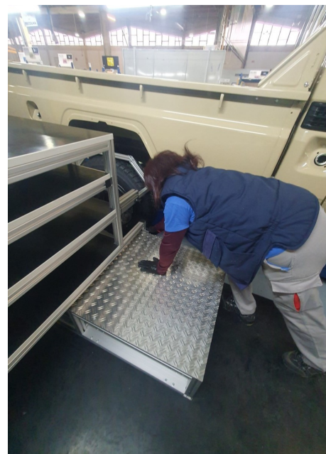
Figure C.27: Step locking system, before - Ergonomic risk
