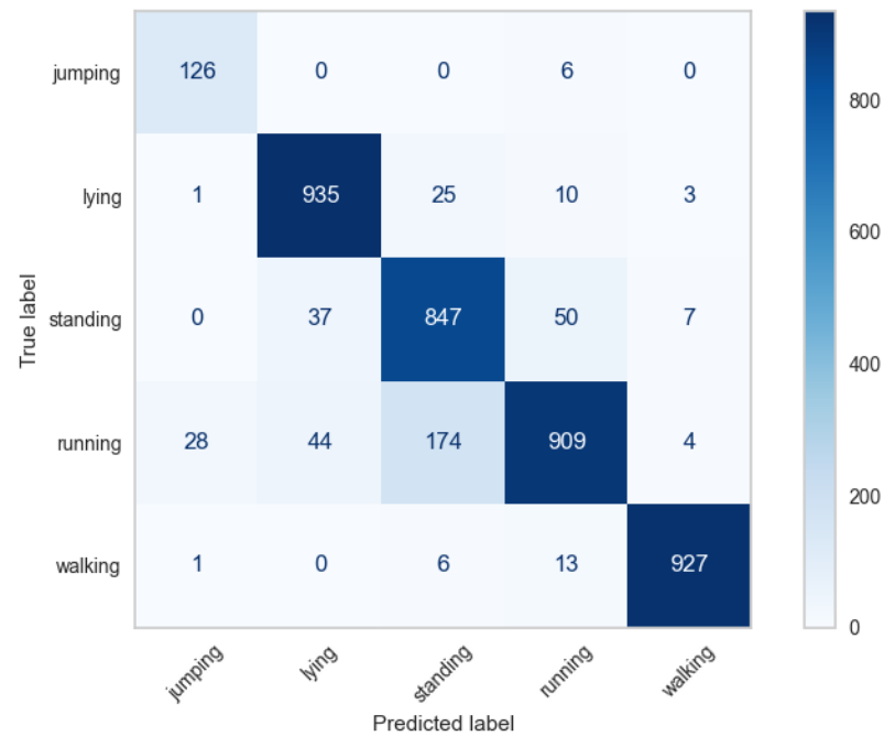
Figure 5.7: Confusion matrix for the RWHAR dataset after hyperparameter tuning for the test data.
