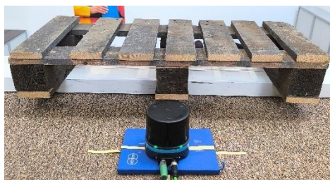
Figure 5.3 - Experimental setup: test pallet and multiScan positioning
