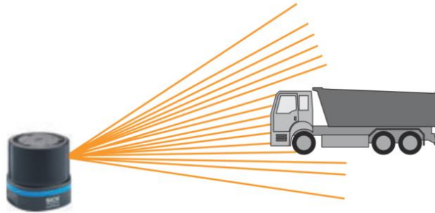
Figure 3.1 - Device with 16 scan layers, side view [12]
