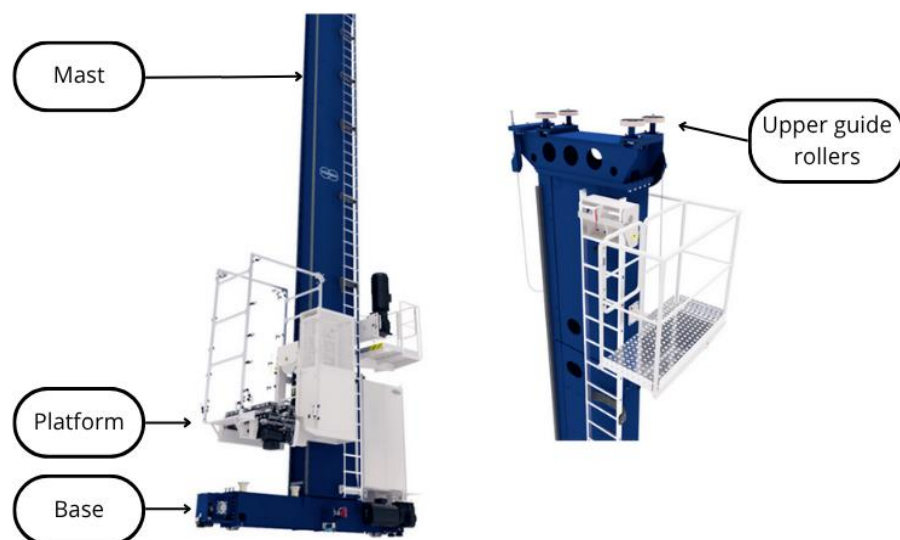
Figure 2.3 - Main Structural Components of the SRM [4]
