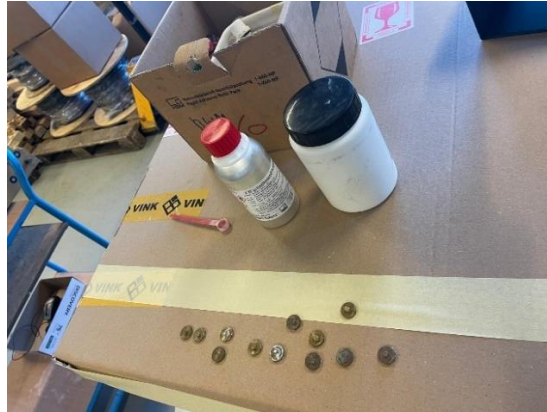
Fig. 4 – X60 adhesive and metal mounting plates used for sensor installation.
