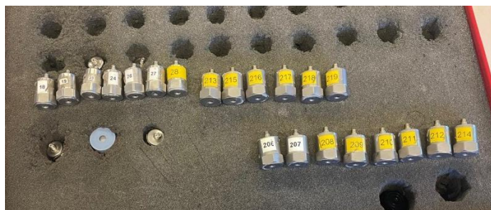
Fig. 5 – Piezoelectric accelerometers used to measure structural vibrations.
