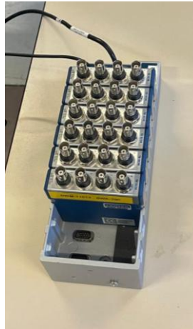
Fig. 6 – National Instruments CompactDAQ system, model cDAQ-9178, used for data acquisition.
