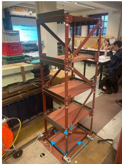
Fig. 2 – Laboratory Frame Structure.
