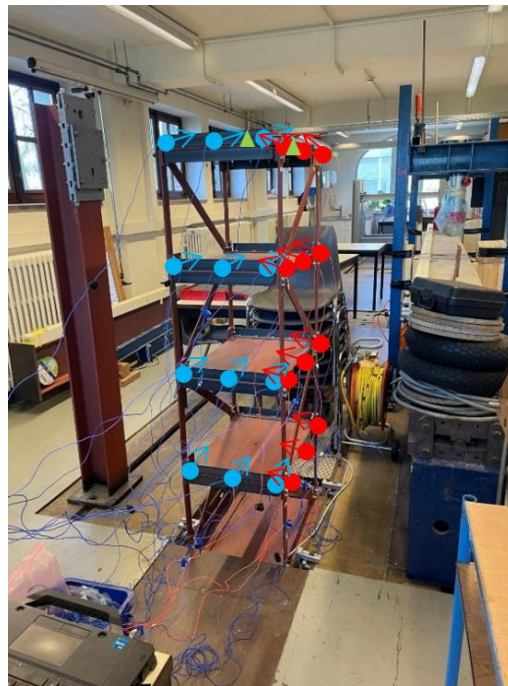
Fig. 7 – Overview of the experimental setup, including sensor positions and excitation points.
