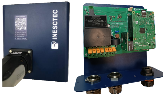
Figure 3.5: INESC TEC's previous IEC 61851-compliant charger.
