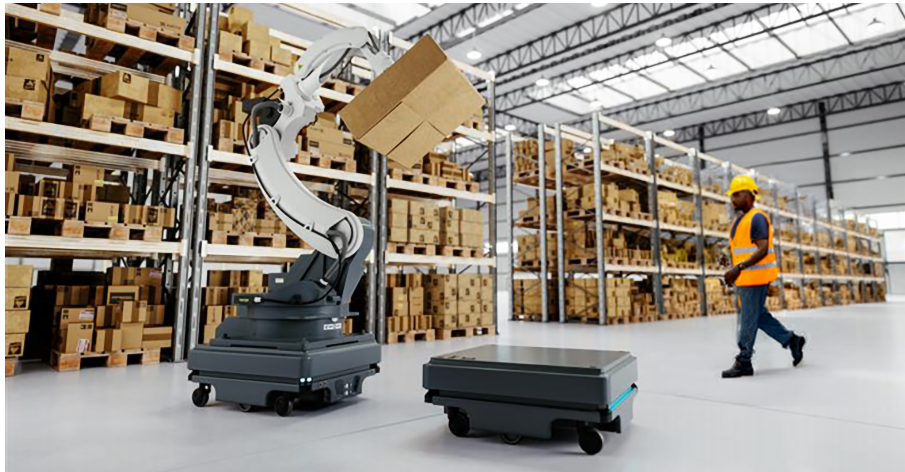
Figure 1.3: An example of a robot as safety-critical system. In human-robot interactions, operation must ensure that no harm is caused to humans or to equipment. Source: https://www.roboteq.com/applications/all-blogs/ .
